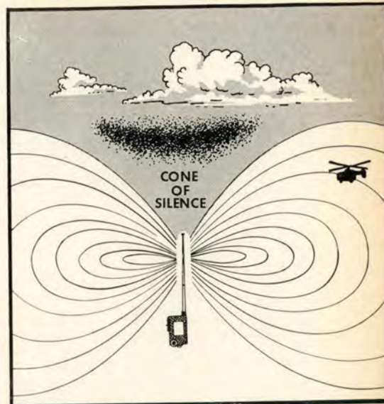
ANTENNA PATTERN FOR URC-10 (RT-10) SURVIVAL RADIO (NOT TO SCALE)
